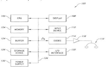
The buffer 124 has a "lockable feature" for limiting the amount of compressed digital data that can be reloaded into the buffer 124 to reduce the frequency in which the storage device 126 has to be activated and the motor therein operable.
