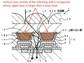
Collabo supplied the following drawing (Collabo's annotations of Abe's FIG. 3), showing the absence of a top and being in a cup-shaped structure, and therefore, <u>not</u> a trapezoid structure for the claimed reflecting wall:
